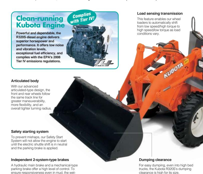
discs are completely sealed and protected.
